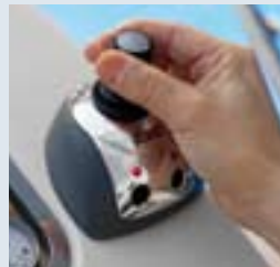
Twist the top to rotate. Combine it with any other move to compensate for wind or current.
