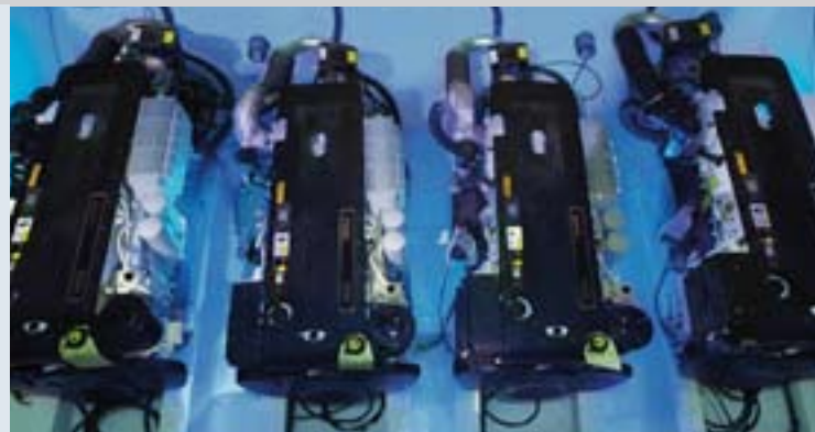
Quadruple installation of Volvo Penta IPS600.
